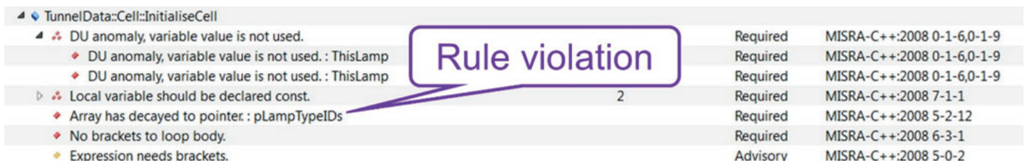
Figure 7: Highlighting violated coding rules and guidelines in the LDRA tool suite
